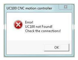
The following popup screen appears if Mach3 loosing the connection with the UC100 meanwhile it is operating. This event may happen if the USB cable is broken or if the cable connector was accidentally slipping out from the UC100 or from the PC. The workaround is checking the USB cable connections and plug it back and restart Mach3.
